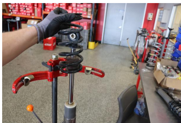
Step 10. Remove OE secondary spring.
