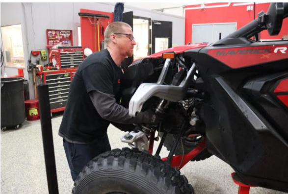
Step 17. Install shock in vehicle between upper and lower control arm.
