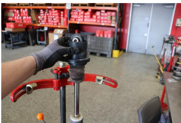
Step 9. Remove spring slider.
