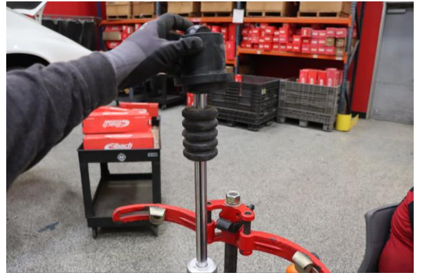
Step 14. Reinstall OE spring slider.
