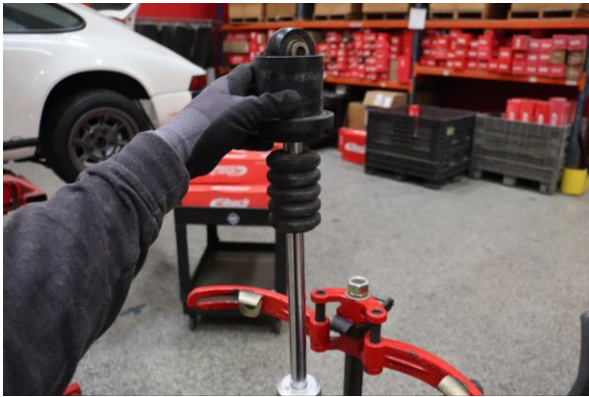
Step 9. Remove spring slider.
