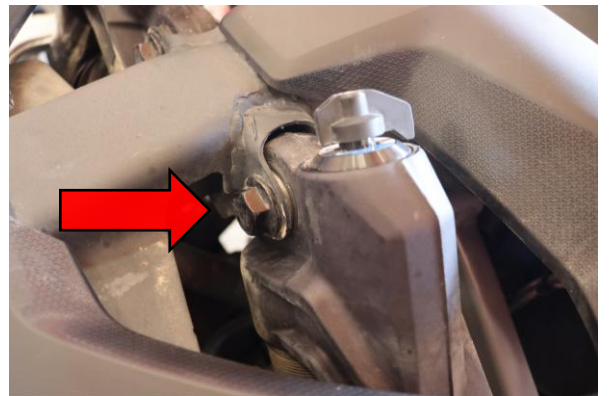
Step 18. Install upper shock mounting bolt to hold shock.
