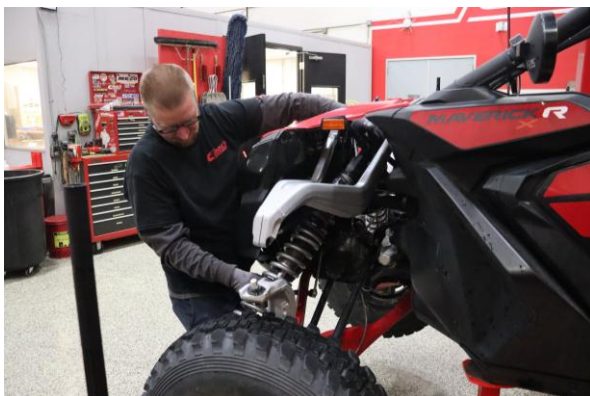
Step 5. Remove shock assembly from vehicle between upper and lower control arms.
