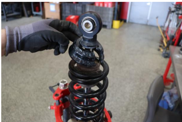
Step 7. Remove the spring retainer.
