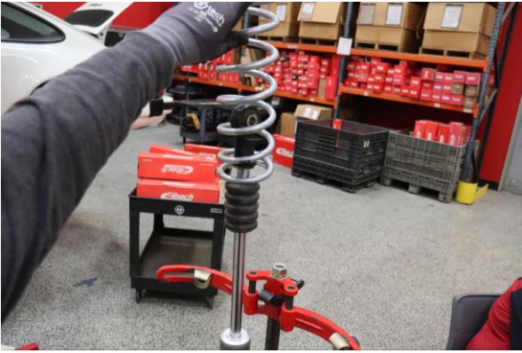
Step 13. Install Eibach secondary spring.
