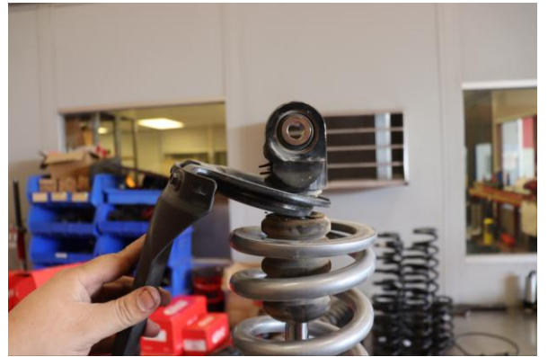
Step 16. Install lower spring retainer. Decompress spring assembly making sure that lower spring retainer and main spring sit flush with lower shock mount.
